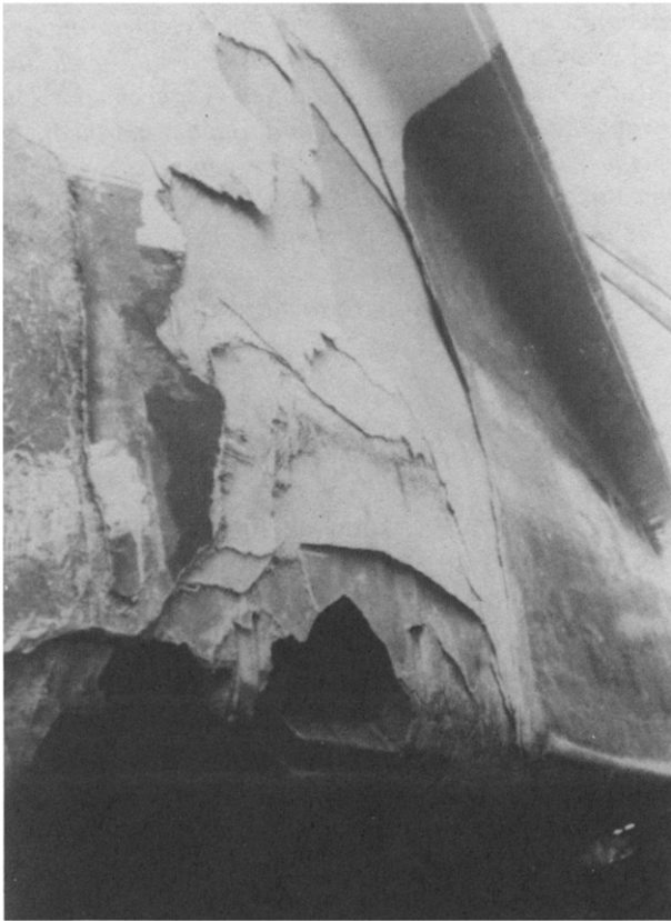
Fig. 2. Damage of a fishing boat due to wave impact—example 2.
